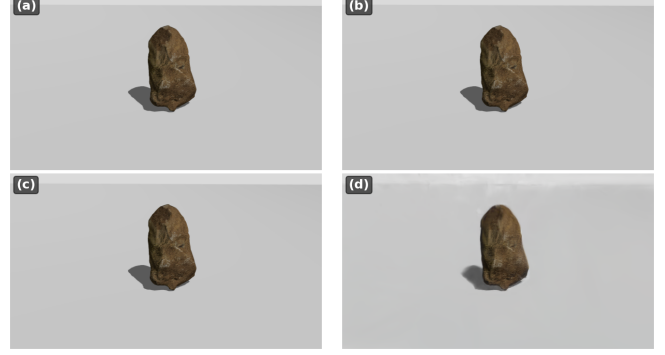
Fig. 4. Qualitative comparison on frame kf_0041 . (a) Ground truth. (b) D-Optimal NBV (54 images, PSNR=28.50 dB, SSIM=0.9530). (c) Coverage-Greedy (50 images, PSNR=26.90 dB, SSIM=0.9480). (d) Original 3DGS trained on all 100 images for 15k iterations (PSNR=34.63 dB, SSIM=0.9792). Note that (d) is evaluated on a training frame and reflects memorisation rather than generalisation.
